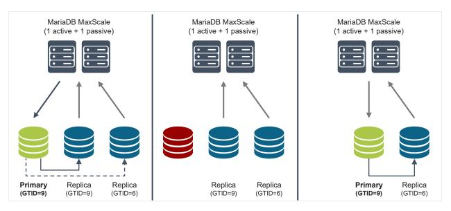
Note: MariaDB MaxScale should be deployed in an active/passive configuration with two instances to ensure high availability and prevent it from being a single point of failure. Further, semi-synchronous replication should be used to prevent data loss in the event of an automatic failover.
